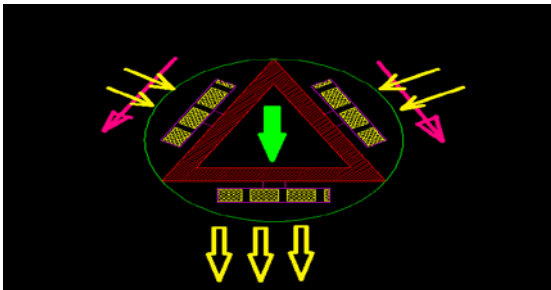
Figure 15. Triangular structured Omni Directional Mobile Robot- Back movement and rotation of wheel and roller directions
